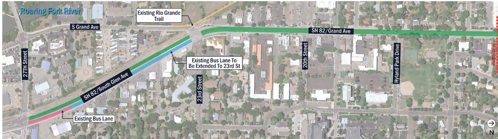
FIGURE 50 - GRAND AVENUE SEMI-DEDICATED BRT LANES PLAN VIEW
