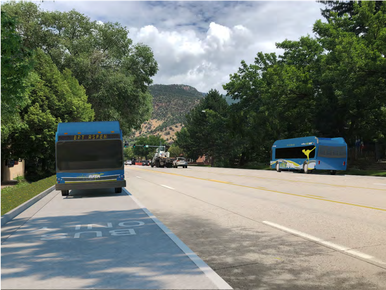
FIGURE 2. GRAND AVENUE SEMI-DEDICATED BRT LANES THAT ALLOW RIGHT TURNING VEHICLES
