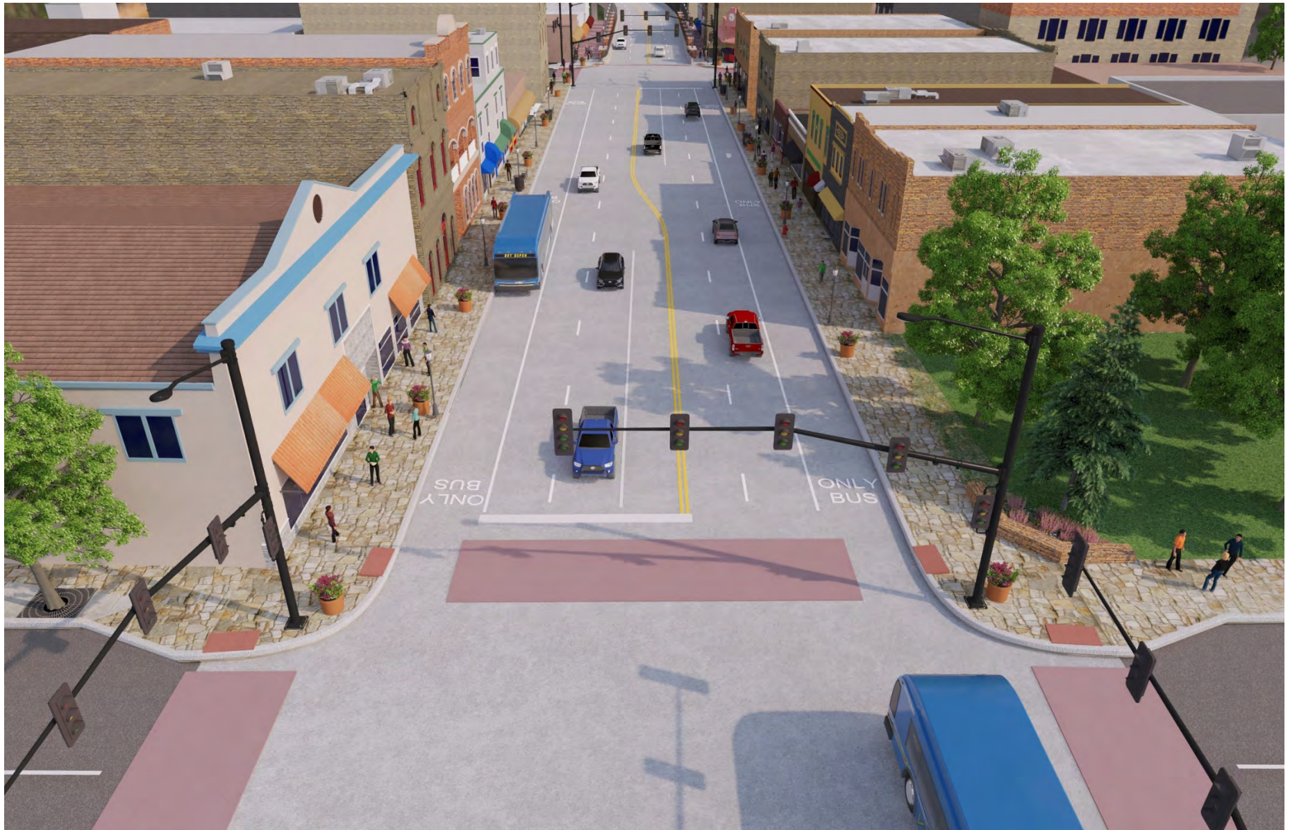
FIGURE 21. GRAND AVENUE SEMI-DEDICATED BRT LANES - TO ACCOMMODATE WIDER LANES NEEDED, THE CURB WILL RECEDE BY 2' RESULTING IN THE REMOVAL OF MATURE TREES AND BULBOUTS
