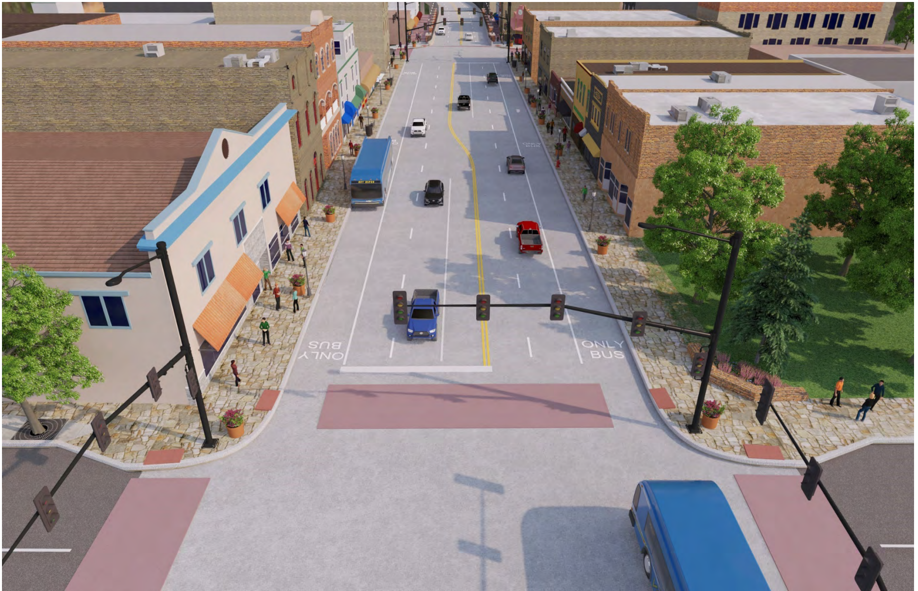
FIGURE 4. GRAND AVENUE SEMI-DEDICATED BRT LANES - TO ACCOMMODATE WIDER LANES NEEDED, THE CURB WILL RECEDE BY 2' RESULTING IN THE REMOVAL OF MATURE TREES AND BULBOUTS
