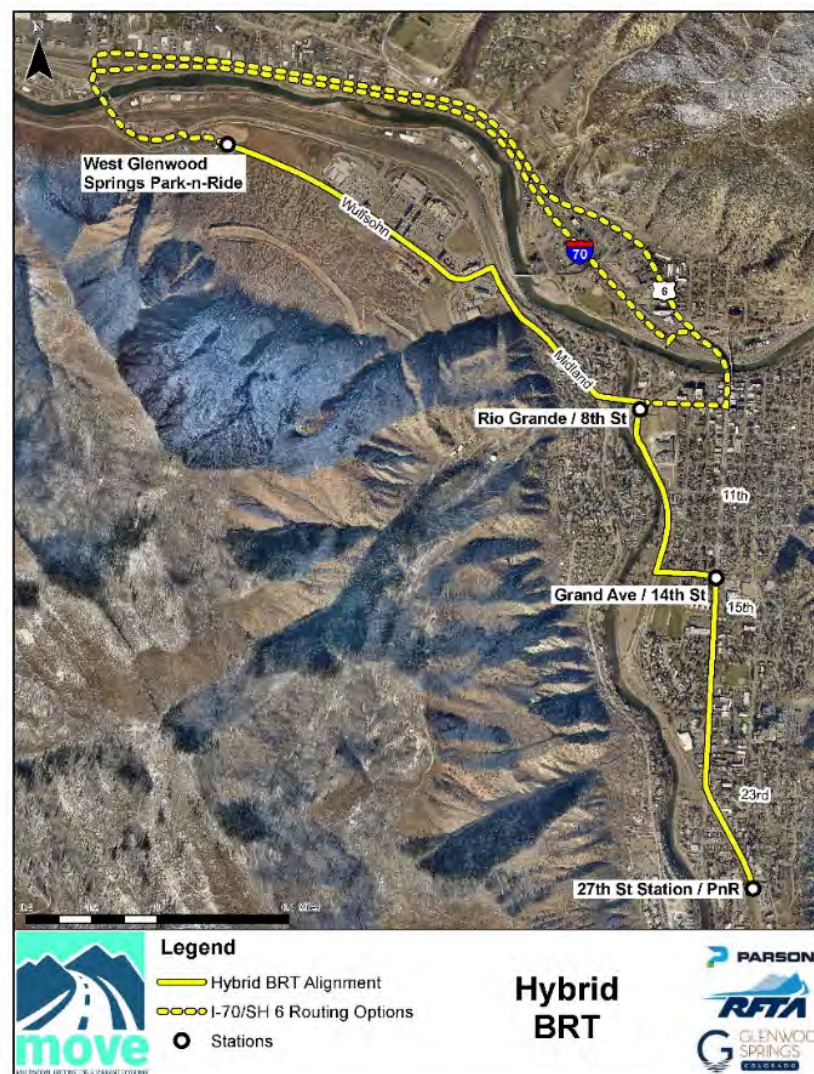
FIGURE ES-2 - HYBRID BRT EXTENSION ALIGNMENT ON GRAND AVENUE AND RIO GRANDE CORRIDOR -
