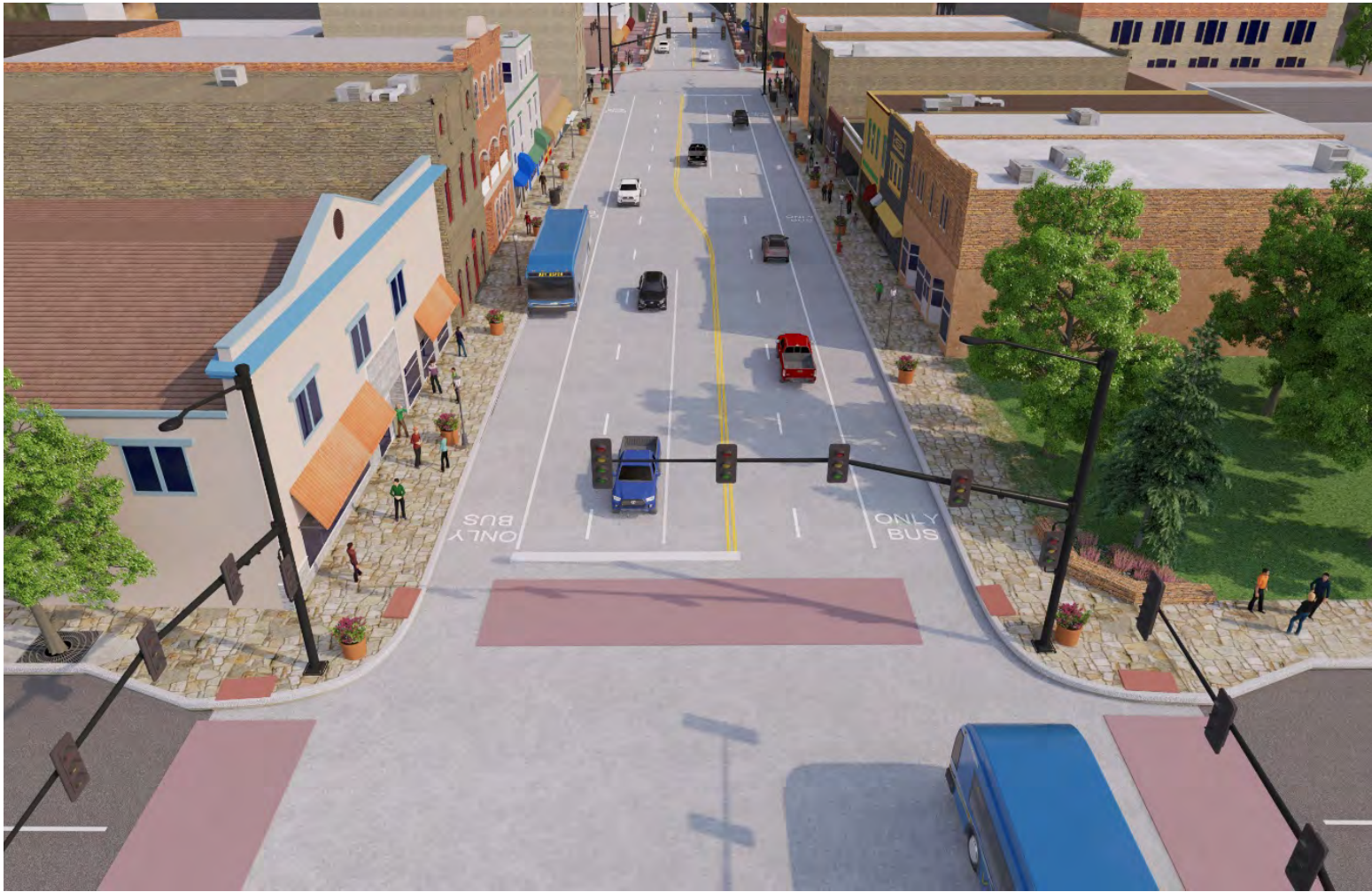
FIGURE ES-3. CROSS SECTION RENDERING OF GRAND AVENUE SEMI-DEDICATED BRT LANES
